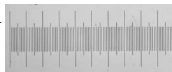
Figure 3. LECO Part No. 860-256-110 Traceable Metric Stage Micrometer (Smallest division 0.01 mm)
