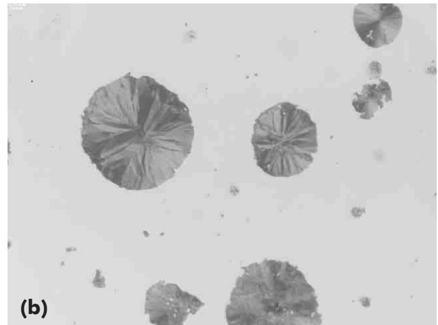
Figure 5: Nodular Cast Iron (a) As-Polished, 500x, (b) As-Polished, under Polarized Light, 500x.
